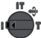
**The Vario-Lock position to change the position of the chisel.** In this position, the rotation shock/stop switch (10) does not engage.
