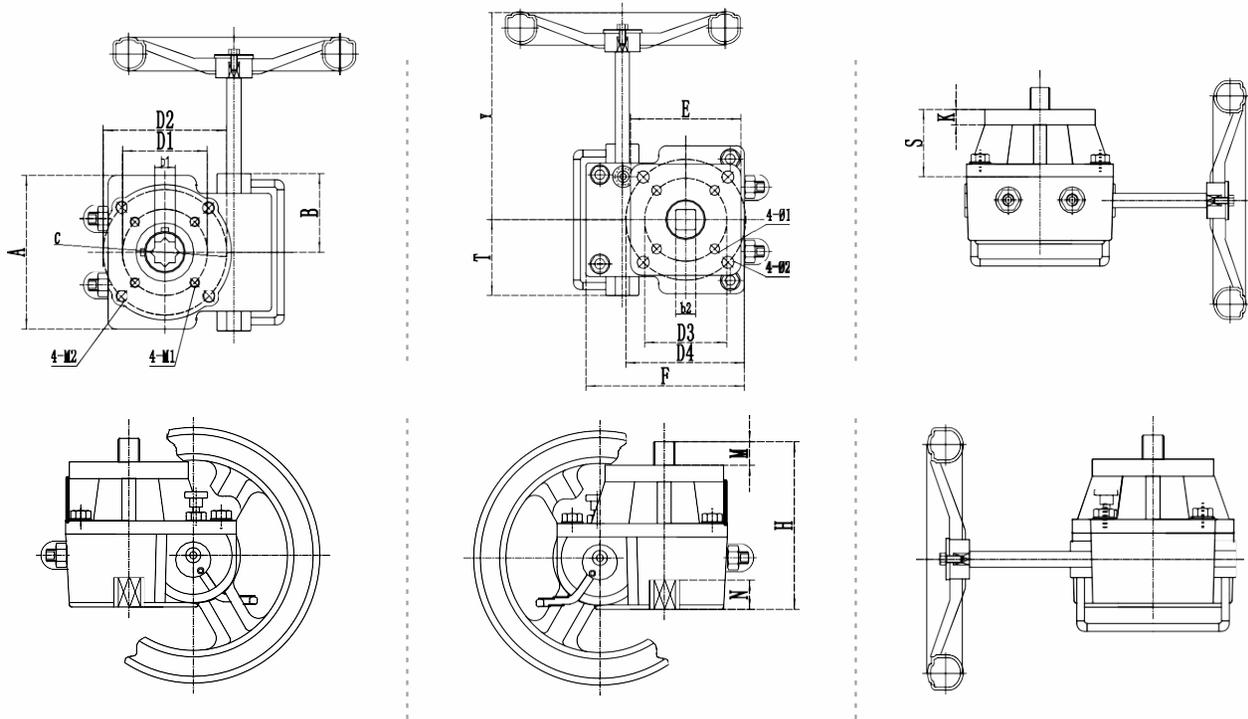
**Remark:**The bottom center of the HDM-4 is either F10/F14 or F10/F12
